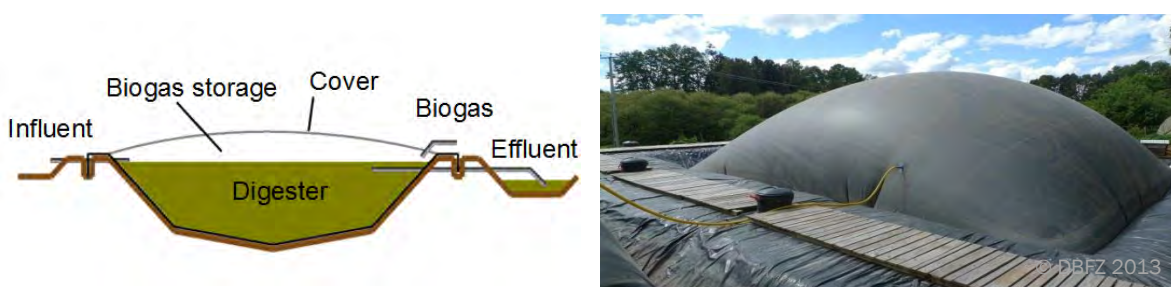
Figure 8.3 "Covered lagoon". Left: Schematic layout. Right: Plant (DBFZ 2013)
