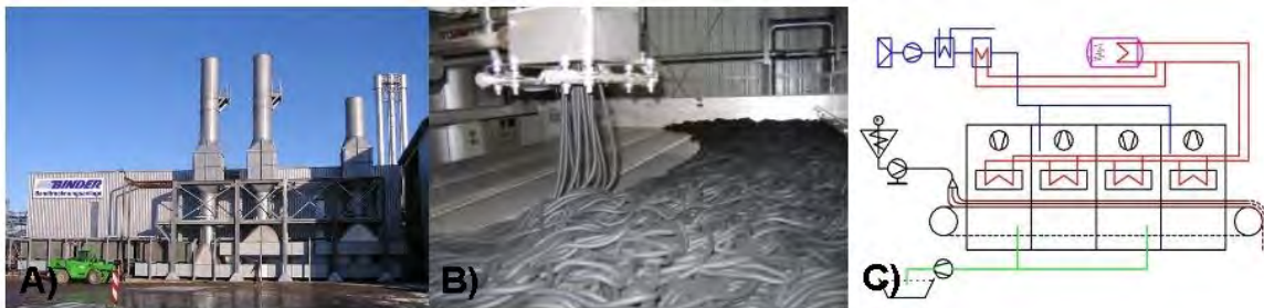
Figure 3.5 Conveyor dryer: A) Overview; B) Product feeder module with extruder; C) Schematic diagram; (by courtesy of Hans Binder Maschinenbau GmbH 2013)
